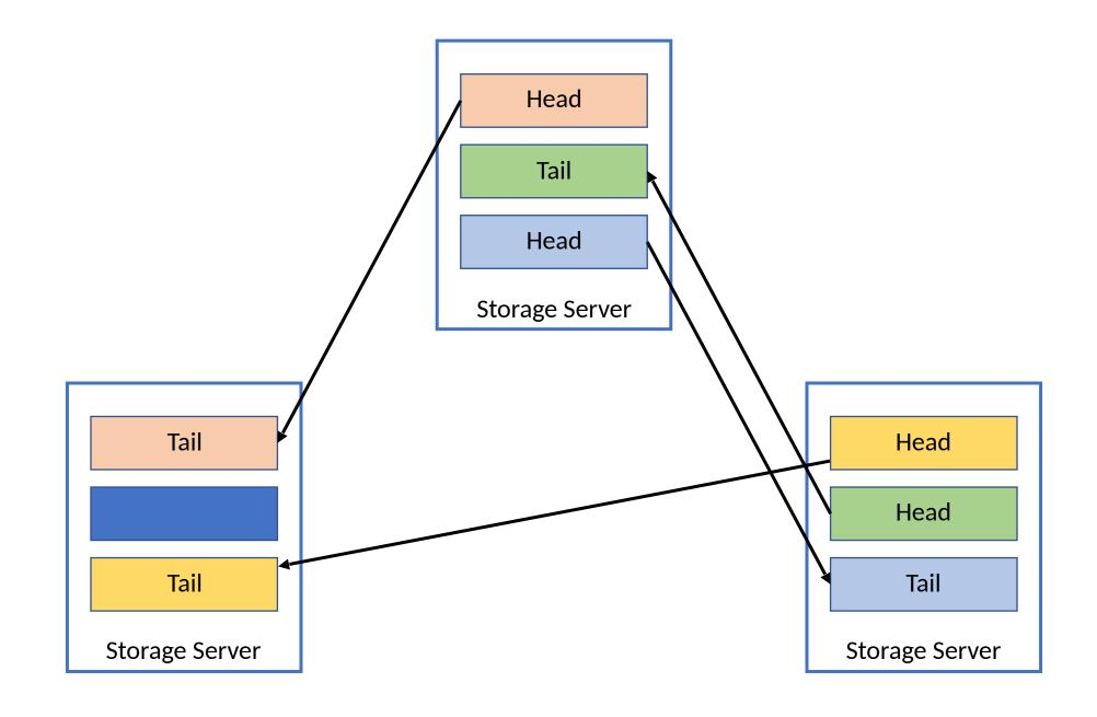
In response to detecting the failure of a server that is part of a chain..., the chain is reconfigured to eliminate the failed server. For this purpose, we employ a service, called the master.
